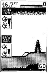
To increase the sensitivity level, press the key adjacent to the menu's up arrow on the left side of the unit. As you press the key, the menu's bar graph will grow taller and the percentage will increase in value. You can also see the difference on the chart record as it scrolls. When the sensitivity is at the desired level, release the key.
